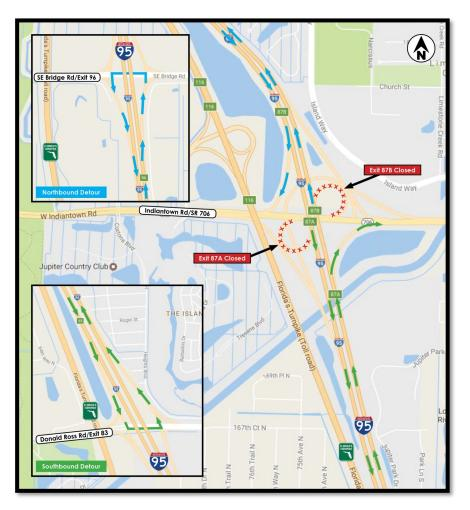
Road 706) to Bridge Road (County Road 708). Work on this project includes: resurfacing I-95 mainline from south of Indiantown Road (SR 706) to north of Bridge Road (CR 708) and the I-95 interchange ramps at Indiantown Road (Exit 87) and Bridge Road (Exit 96), and minor shoulder and guardrail repairs.
